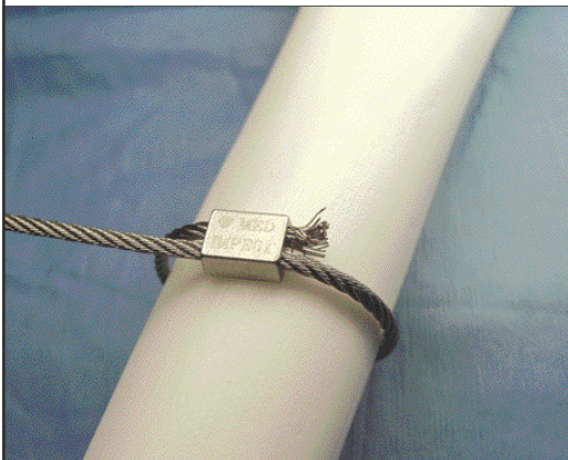
Trimmed or broken ends of wire cerclage cables fray and can irritate patient tissue. These sharp ends also pose a safety hazard to surgical teams.
