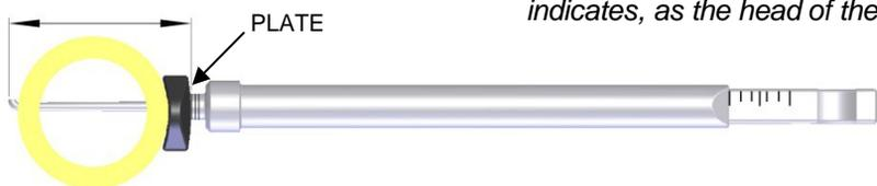
*Depth gage reading indicates distance from the top of plate to the tip of gage*
