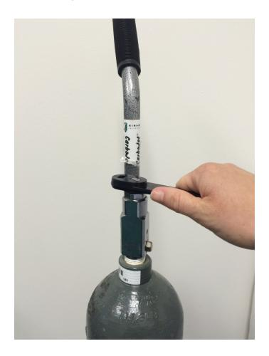
CAREFULLY open the cylinder valve a very small amount for only an instant. Then close the valve quickly to blow out any foreign matter in the valve port.
