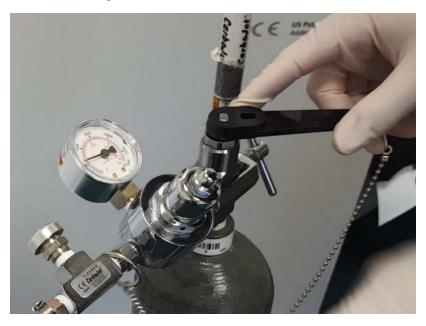
**VERY IMPORTANT:** After the surgery is completed, double check that the cylinder valve is completely closed prior to the removal of the regulator from the cylinder. The regulator may be left in place on the  $CO_2$  tank so that it is ready and available for use on the next case.
