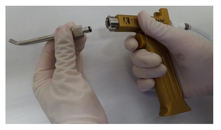
Select a nozzle and attach it to the nose of the handpiece via the quick disconnect fitting. Push the nozzle into the fitting until it clicks in place.
