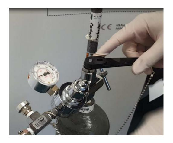
Following *CarboJet* use, close the valve on the CO<sub>2</sub> tank and purge the *CarboJet* System by depressing the handpiece trigger.
