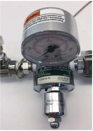
The *CarboJet* pressure regulator should be inspected for damage, dirt, dust, oil, or grease. Remove dust or dirt with a clean cloth. Do not use the regulator if oil, grease, or damage is present. No other maintenance is required for the regulator, except as described on Page 12. The regulator is used outside of the sterile field and should not be sterilized.
