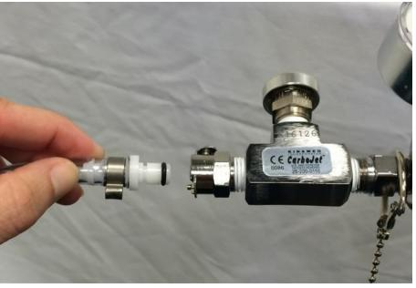
Open the pouch containing the sterile tube set and deliver the contents to the sterile field. Using the white quick disconnect fittings at each end of the tube set, connect the female end of the tube set to the handpiece and then pass the male end of the tube set out of the sterile field and connect it to the pressure regulator.
