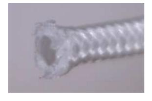
4. Use light finger pressure to slide the sheath over the end of the nylon by ¼ inch (6mm).
