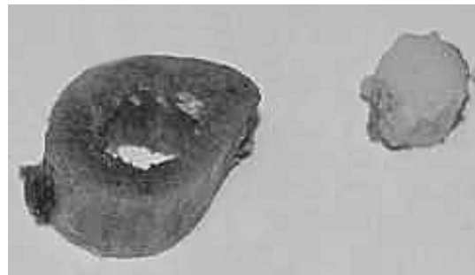
Fig. 2 Cement extrusion with an intact cortical rim. This mode of failure was seen in specimens prepared with saline irrigation.
