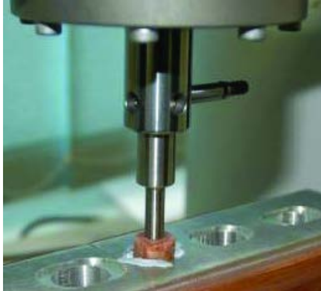
Fig. 1 Apparatus set-up with instrom machine used to push cement out of cortical sections.
