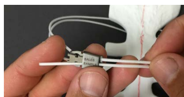
B. Feed cable strands through locking clasp.
