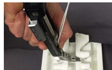
G. Hold cable strands over cleats with thumb or finger and begin to tension cable by turning knob clockwise.
