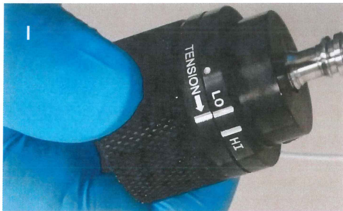
1 st mark indicates 80 lbs (360 N) compressive force.
