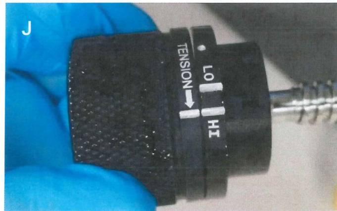
2 nd mark indicates 120 lbs (530 N) compressive force.
