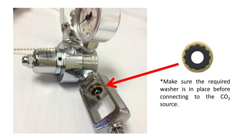
All regulators used with cylinders/tanks come fitted with an appropriate washer.
