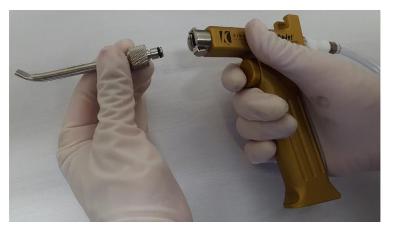
Select a nozzle and attach it to the nose of the handpiece via the quick disconnect fitting. Push the nozzle into the fitting until it clicks in place.
