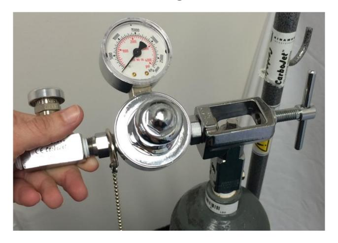
Install the pressure regulator to the CO<sub>2</sub> cylinder/source making sure it is securely fitted.
