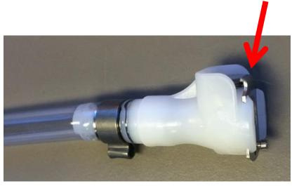
Both tubing end fittings are simply pushed into place until an audible click is heard. If the quick disconnect fittings do not "click" into place, reset the spring loaded actuator on the corresponding mating fittings (see arrows above).
