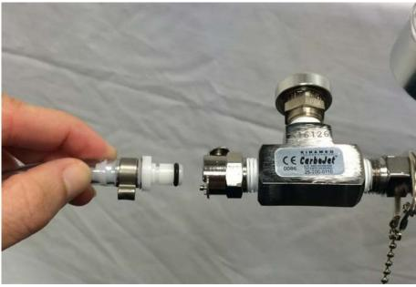
Disconnect the tubing from the regulator and handpiece. Discard the used tube set and any disposable nozzles. Tube sets and disposable nozzles cannot be re-sterilized and are not reusable.
