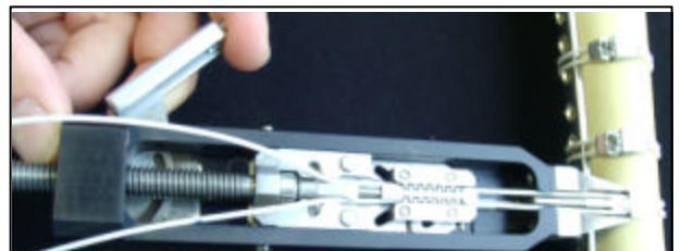
Figure 10B. Re-seat locking wedge before trimming free cable ends.
