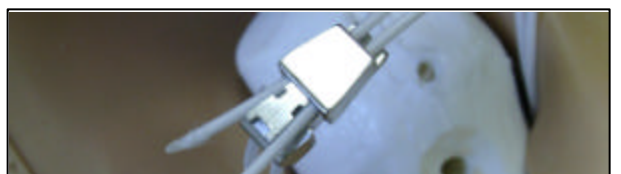
Figure 4B. Feed cable ends through metal clasp.
