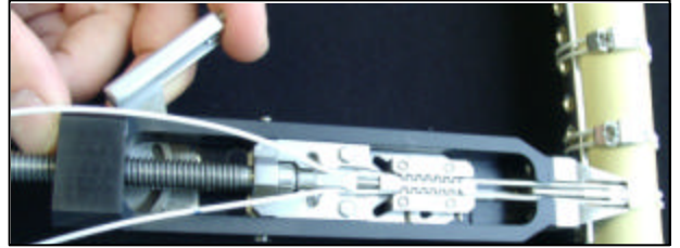
Figure 8. Activate wedge inserter.
