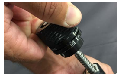
H. Observe tension reading while slowly turning knob.
