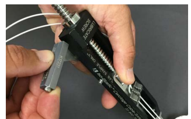
I. Pull back on lever until it stops to fully seat locking wedge.
